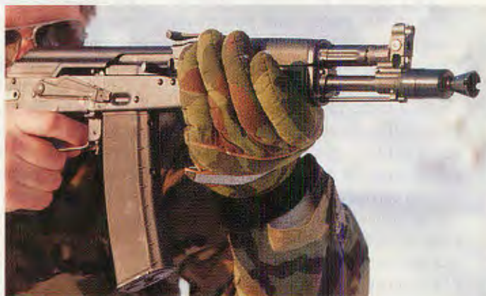
All rifles in the AK100 series have cyclic rates of 600 rpm, which permit operators to consistently fire two-shot bursts with a minimal amount of training. This technique provides maximum hit probability in the full-auto mode.
